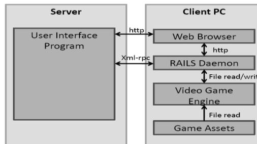
Fig.2. Simplified RAILS Software Component Interaction Diagram
