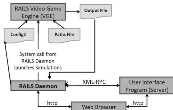
Fig. 3. Diagram Depicting RAILS Software Component Interactions.
